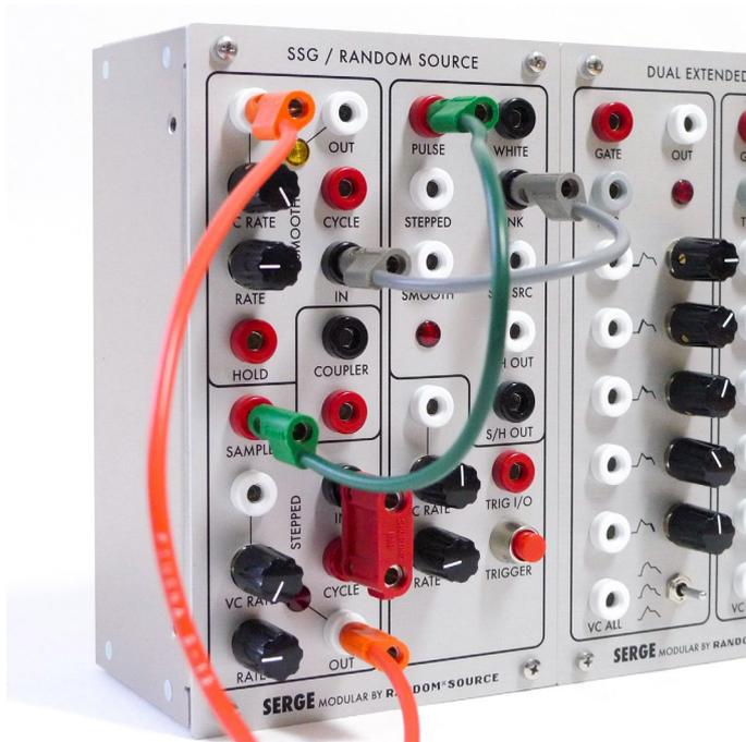
Technically, the Random Source is a combination of a Serge Smooth & Stepped Generator (SSG) with the Noise Source module. The Random\*Source edition combines both modules on one single pcb, so that no stacking of pcbs is required any more. The Random\*Source version of the Random Source is a licensed and authorized adaption of the original Serge designs.
